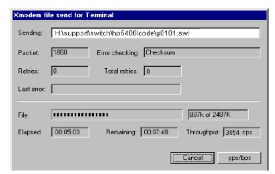
When the download completes, the switch reboots from primary flash using the OS image you downloaded in the preceding steps, plus the most recent startup-config file.
